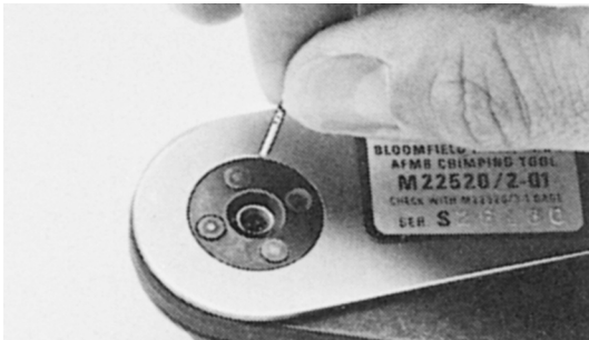
3 - Insert the contact in the crimping tool
