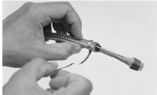
2 - Slide the shielded braid over the chimney as well as the 3 mm "band it" ring.
