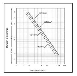
**Note** The above data are average values, and can be obtained within 3 charge/discharge cycles. These are not minimum values.
