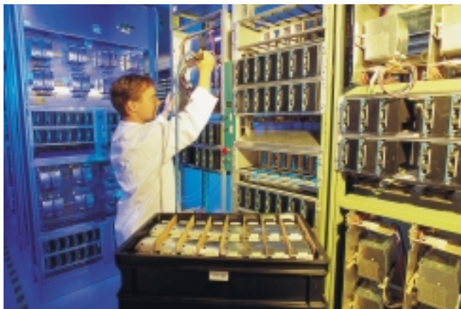
All Allen-Bradley power supplies are burn-in tested to ensure reliability during system start-up.
