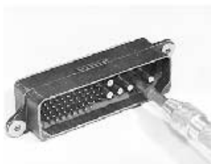
Extracting Coaxial & #12 Contacts
