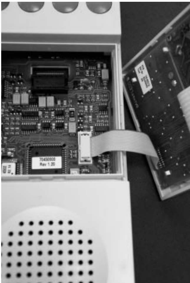
Communication-Terminal: Connection of Mother- and Daughter-Board with ODU MINI-FIX
