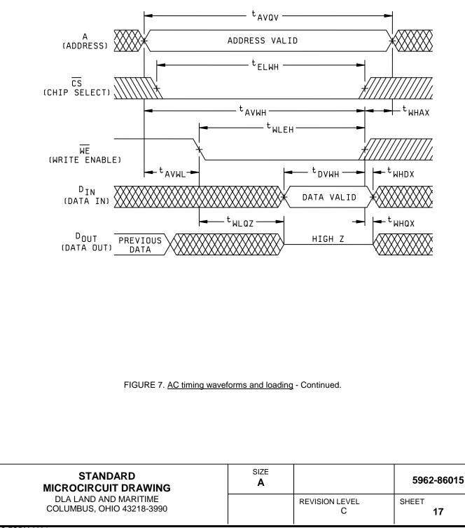
Write cycle 2. This write cycle is  $\overline{CS}$  controlled, where  $\overline{WE}$  is active (LOW) prior to or coincident with  $\overline{CS}$  becoming active (LOW). In this write cycle the data out remains in the high impedance state (3 state) at the beginning of the write cycle, precluding potential data contention in common I/O application.
