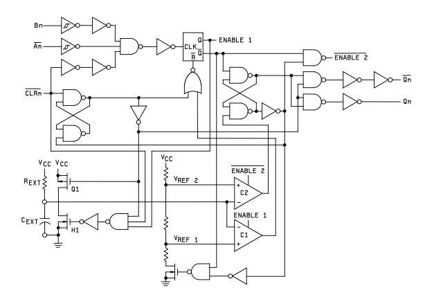
FIGURE 3. Logic diagram.
