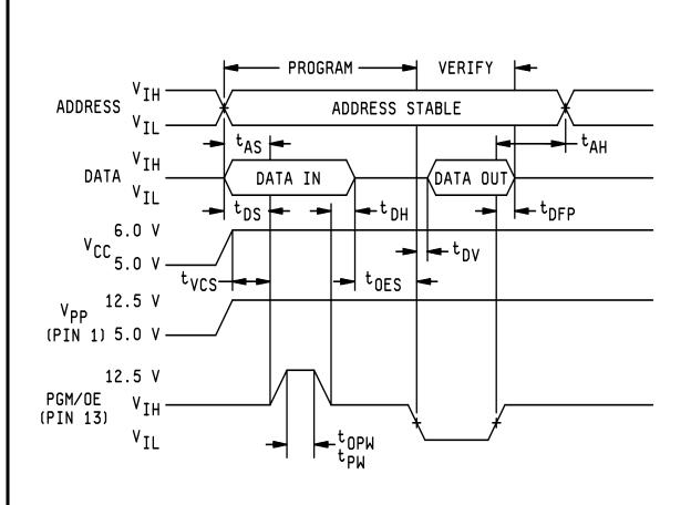
FIGURE 6. Programming waveforms.
