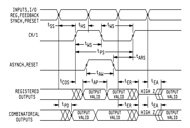
NOTE: Timing measurement reference is 1.5 V. Input ac driving levels are 0.0 V and 3.0 V, unless otherwise specified.
