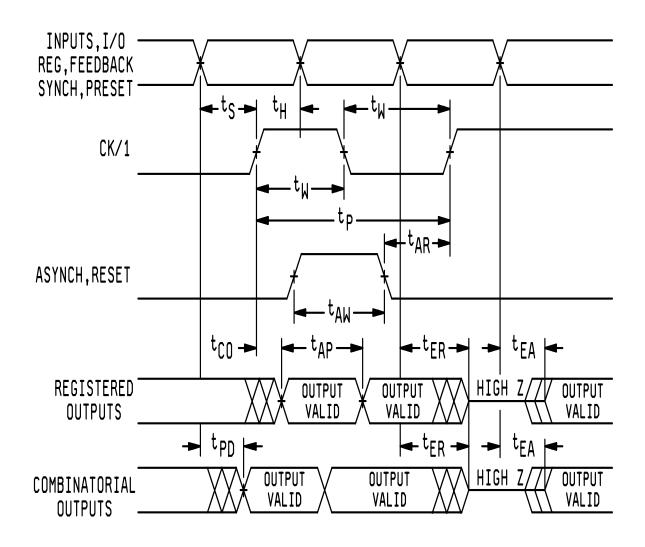
NOTE: Timing measurement reference is 1.5 V. Input ac driving levels are 0.0 V and 3.0 V, unless otherwise specified.
