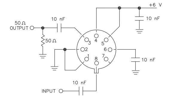
FIGURE 3. Test circuit.
