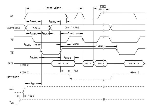
NOTE: RDY/ $\overline{\text{BUSY}}$ ,  $\overline{\text{RES}}$ , and V<sub>CC</sub> waveforms are applicable to device types 16-19 only.
