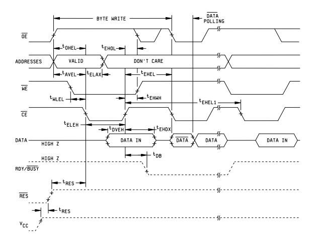
NOTE: RDY/ $\overline{\text{BUSY}}$ ,  $\overline{\text{RES}}$ , and V<sub>CC</sub> waveforms are applicable to device types 16-19 only.
