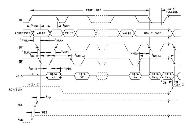
NOTE: RDY/ $\overline{\text{BUSY}}$ ,  $\overline{\text{RES}}$ , and V<sub>CC</sub> waveforms are applicable to device types 16-19 only.
