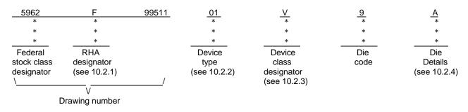
10.2.1 <u>RHA designator</u>. Device classes Q and V RHA identified die shall meet the MIL-PRF-38535 specified RHA levels. A dash (-) indicates a non-RHA die.
