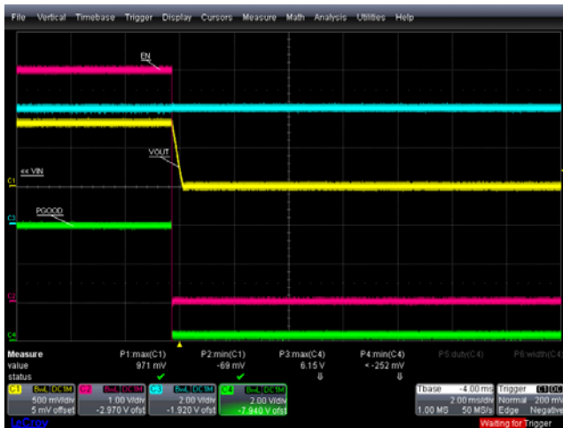
FIGURE 25. POWER-ON AND POWER-OFF, EN = 1 TO 0, +25 °C, VIN = 6V, VOUT = 0.8V, IOUT = 0.5A, PGOOD TURN-OFF
