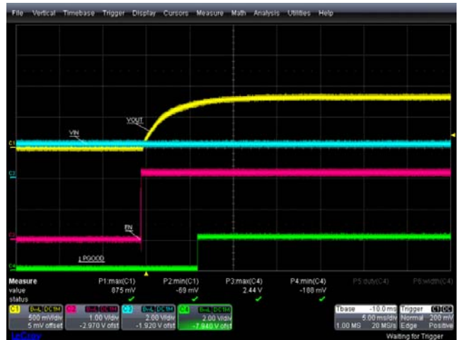
FIGURE 24. POWER-ON AND POWER-OFF, EN = 0 TO 1, +25 °C, VIN = 2.2V, VOUT = 0.8V, IOUT = 0.5A, PGOOD TURN-ON
