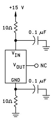
FIGURE 2. Radiation exposure circuit.
