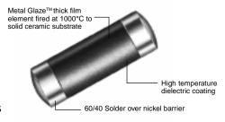
The MCHP High Reliability Surface Mount Resistors are part of the RG product family of precision resistors developed by IRC in 1960 to meet the stringent demands of the military market. In leaded form, these resistors are qualified to level S under MIL-R-39017 and MIL-R-55182. The MCHP resistor utilizes the core element from this series, but with modified contacts and encapsulation.
