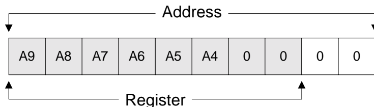
Figure 8-4. FIFO Start Address Format
