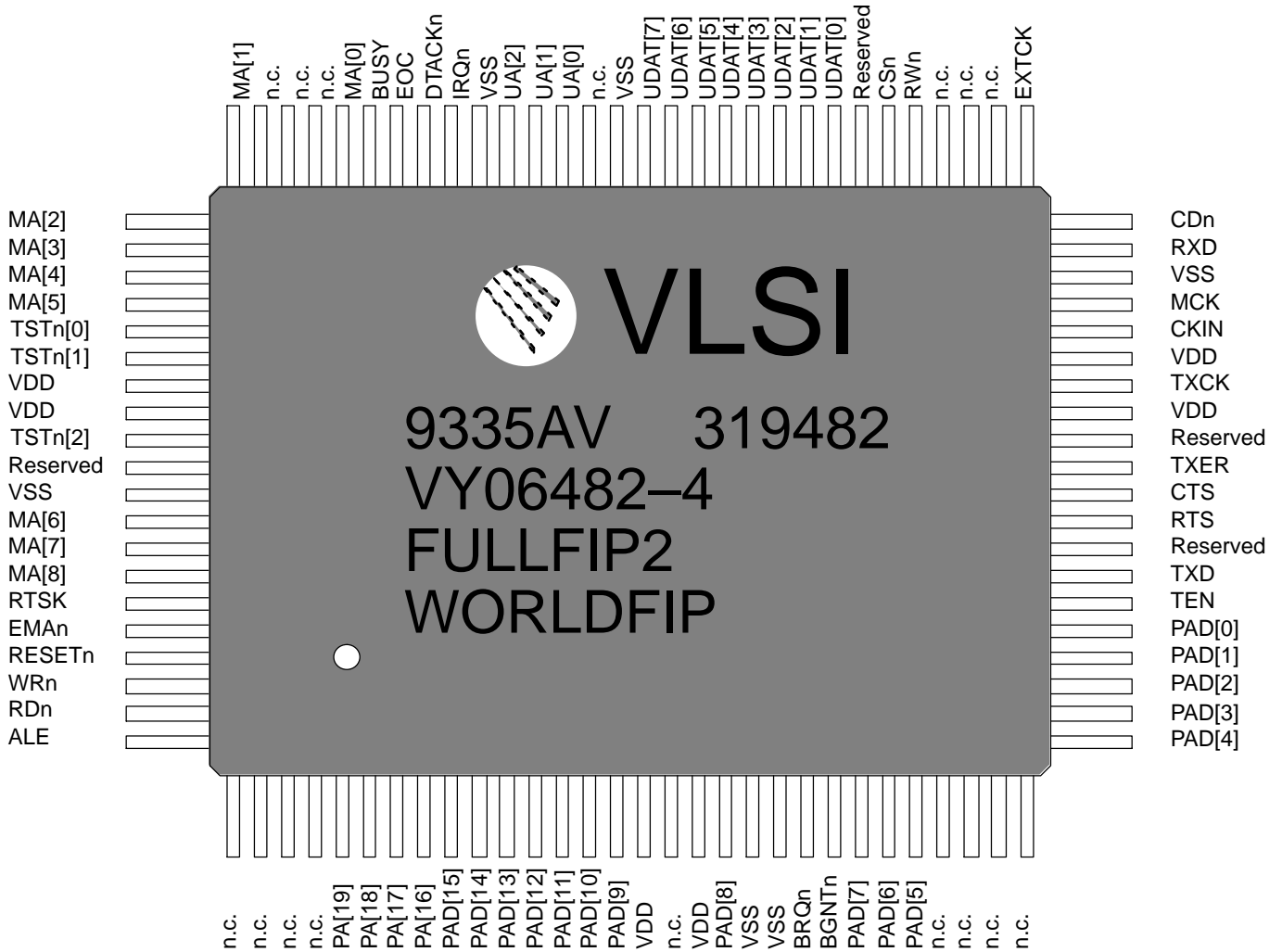
Figure 2.2 – FULLFIP2 pinout diagram – MQFP100 package – Top view
