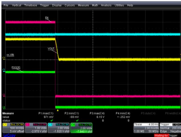
FIGURE 23. POWER-ON AND POWER-OFF, EN = 1 TO 0, +25°C, V_{IN} = 6V , V_{OUT} = 0.8V , I_{OUT} = 0.5A , PGOOD TURN-OFF
