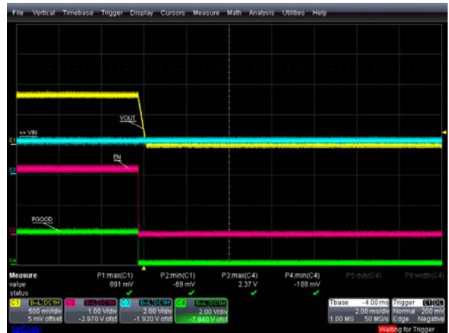
FIGURE 24. POWER-ON AND POWER-OFF, EN = 1 TO 0, +25°C, V_{IN} = 2.2V , V_{OUT} = 0.8V , I_{OUT} = 0.5A , PGOOD TURN-OFF
