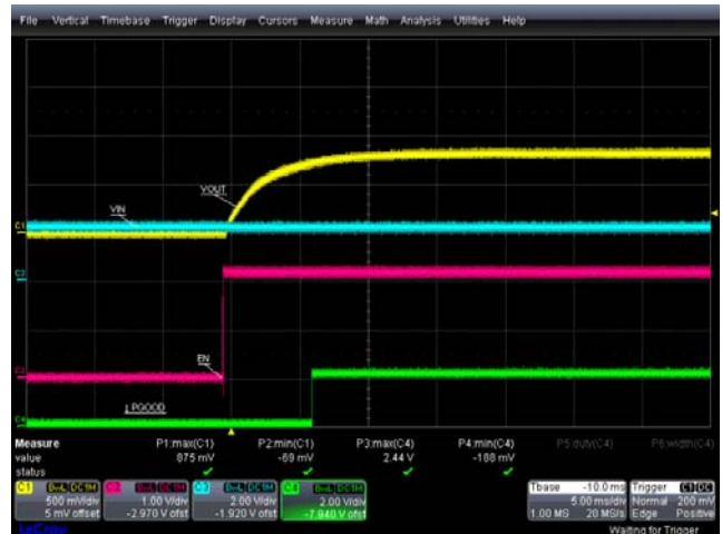
FIGURE 22. POWER-ON AND POWER-OFF, EN = 0 TO 1, +25°C, V_{IN} = 2.2V , V_{OUT} = 0.8V , I_{OUT} = 0.5A , PGOOD TURN-ON
