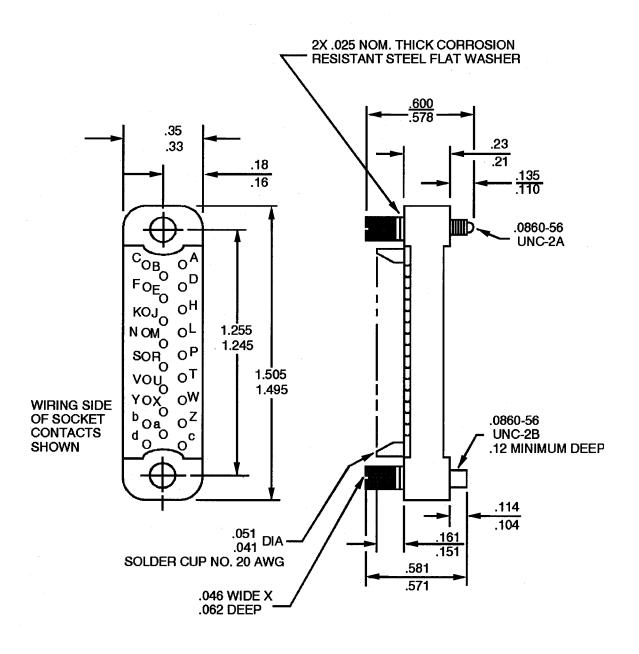
FIGURE 1 - DESIGN AND CONSTRUCTION
