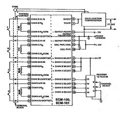
In this application, the SCM-100 is set up as a four-channel thermocouple input system with isolation, amplification, and multiplexing provided by the module. Various thermocouple types are used, and the gain adjust pots on each channel have been selected to take the standard ANSI range for each thermocouple to a 5V output span. A universal cold junction compensator is used to compensate for the temperature of the reference junction which is formed where the thermocouple leads are terminated.
