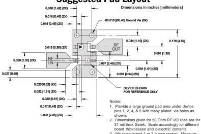
We recommend 1 or 2 ounce copper. Measurements for this data sheet were made on a 31 mil thick Getek with 1 ounce copper on both sides.
