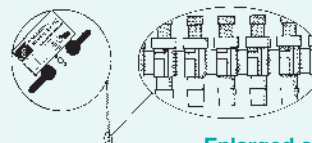
Enlarged section of plastic contact carriers
