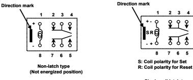
Single coil latch type (Reset position)
