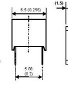
Tolerance of lead pitch is  $\pm\,0.15\text{mm}$  (0.006inch) Other tolerances  $\pm\,0.3\text{mm}$  (0.012inch) NJ type: Lead length 2.8mm
