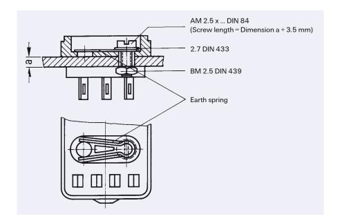
Direct mounting of relays without socket requires a fixing nut M2.5 DIN 934-m6AU. Ordering code: D00934-A0025-S001
