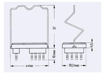
with hold-down spring for cradle relay W
